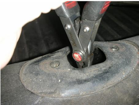
With the shifter removed, pull the shift rod up and down with pliers to check the bushing's condition.
