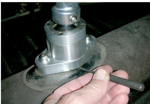
Fine tune the relationship of the shift housing to the guide plate by tapping the plate left or right under the shift housing. Do this operation with the hold down bolts half tight.
