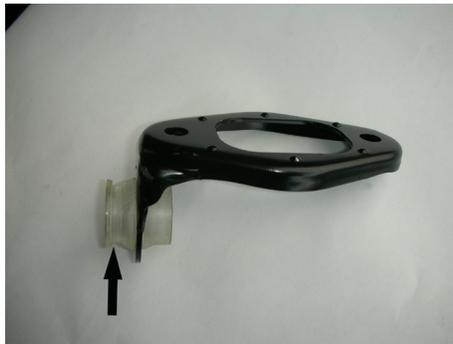
This is a new replacement bracket and bushing. The plastic bushing is available at most stores. We do not recommend using the original VW tension ring which was originally located at the arrow.
